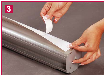
3 Remove the paper backing from the tape on the leader strip.
